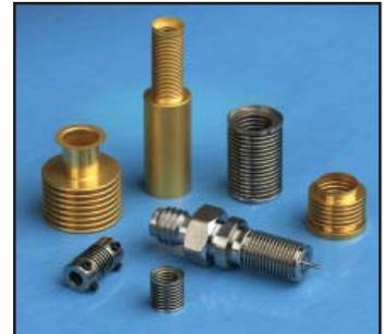
A metal bellows has the physical form of a flexible, spring-like accordion, but once it is filled with a liquid or gas under atmospheric or vacuum conditions and its ends are sealed, the bellows will be extremely sensitive to a variety of forces, providing a predictable, dynamic mechanical response. In vacuum or pressure applications bellows are fabricated as part of sealed, leak-tight assemblies, with appropriate ends to allow connection within the equipment itself.
